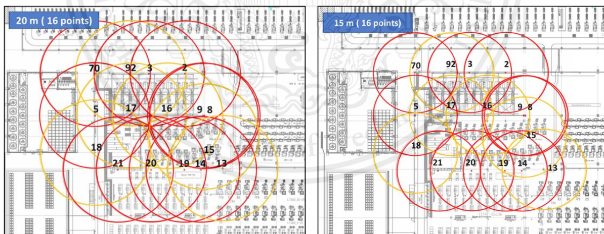
Figure3. 11 Draft a circle of the space to install fire extinguisher in 16 points of fire extinguisher at diameter 15 meters and 20 meters
