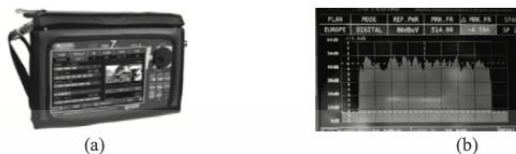
Figure 12 Measurement equipment (a) DVB-T2 analyzer (b) Example spectrum mask of MUX 1.
