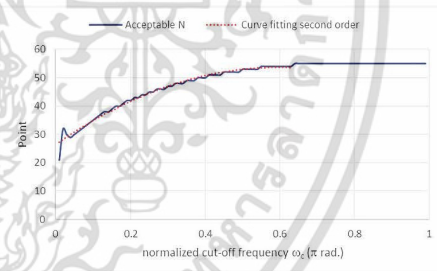
Fig. 4 The relationship of acceptable N and cut-off frequency.
