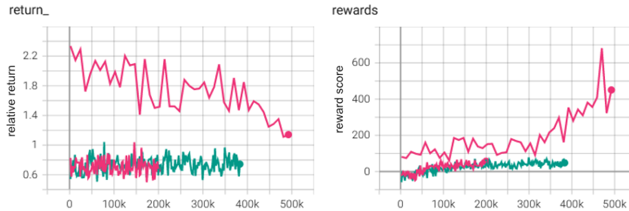
Figure 4.6: Rewards and returns (PPO) when using state space with three values. The declining pink line in return_ , corresponds to the upper pink line in reward , appeared when Sortino is involved in reward calculation. The x -axis indicates the number of timesteps of learning.
