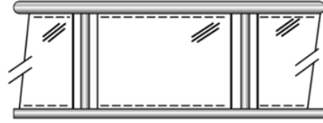
FIG. 2 a Type II: Two-Side Support—Single Lite Glazing as Infill
