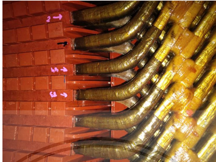
Fig. 2.7 Insulation system in the slot exit area.
