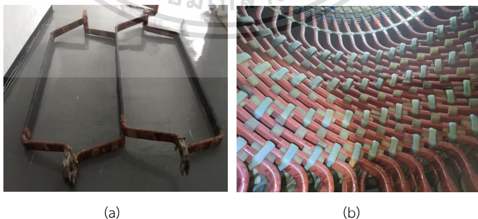
Fig. 2.3 Form-wound (a) stator bars and (b) complete winding.
