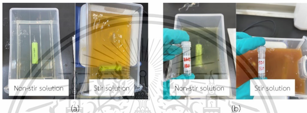
Figure 4.16 Solutions after SSW submersion with and without magnetic stirrer (a) 10 minutes after submersion started (b) 3 hours after submersion started
