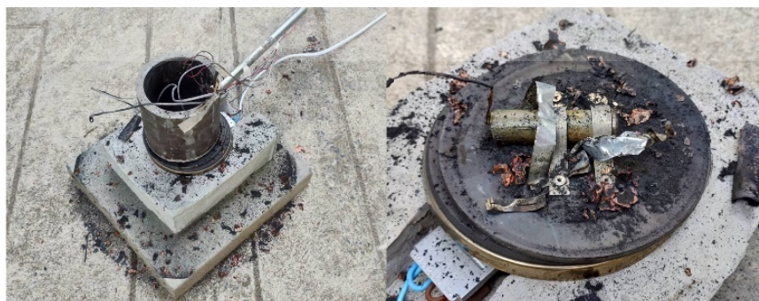
Figure 5.4 Exploded cell after fire and explosion
