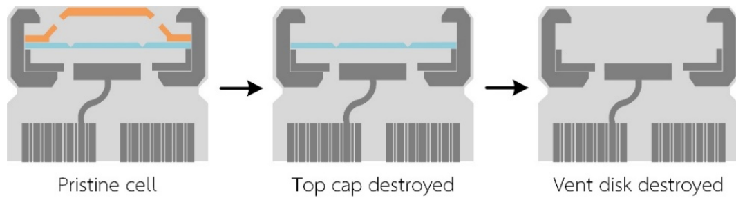
Figure 4.7 Structural collapses of cylindrical LIB during liquid submersion
