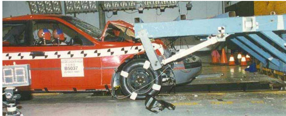
Figure 2.7 Test crash with the RUPD system in the center crash event [9].
