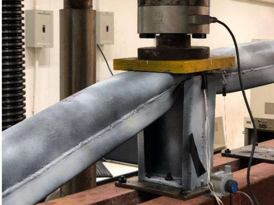
Figure 4.5 Experimental testing of protective beam model result regarding load applied at point P2.
