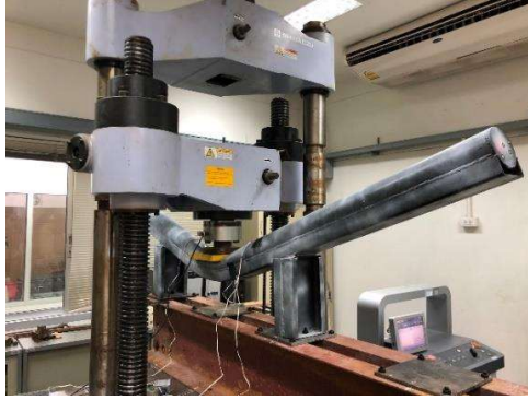
Figure 4.7 Experimental testing of protective beam model result regarding load applied at point P3.
