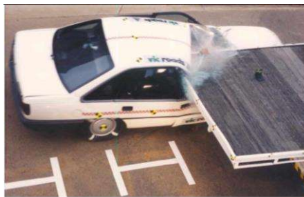
Figure 2.6 Test crash without the RUPD system in offset crash event [9].
