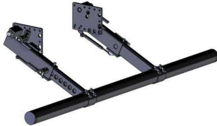
Figure 2.28 WAP Lift-up RUPD with adjustable length legs [12].
