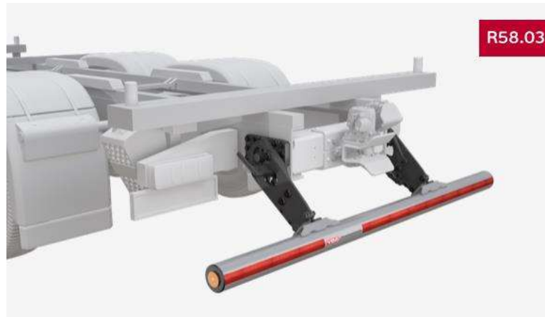
Figure 2.24 VBG foldable RUPD system with cylindrical steel profile [11].
