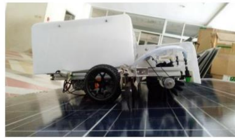
Fig. 8 Robot at various tilt angles on solar cells
