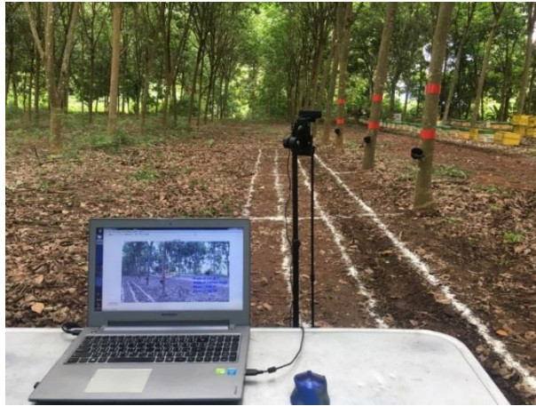
(ก) Two separate targets on each rubber tree in an uncontrolled environment of an actual tree orchard
