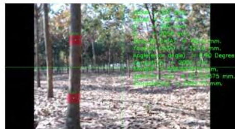
Fig.5 Detection of separate targets on the rubber tree on the uncontrolled environment of actual tree orchard
