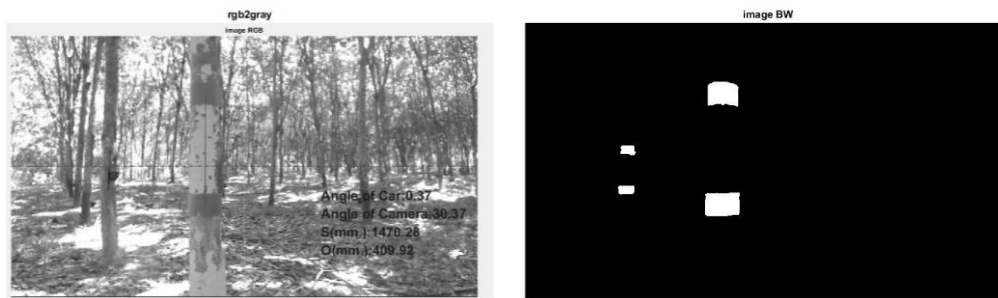
(ค) The grayscale image frame. (ง) The binary image frame.
