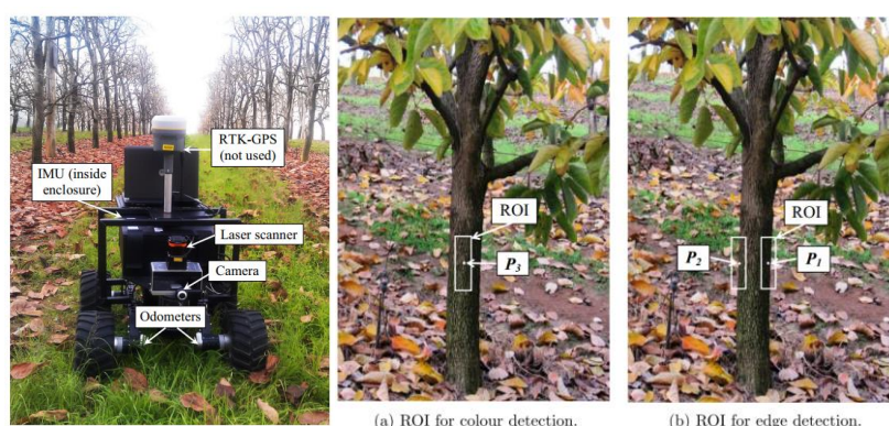
รูปที่ 2.9 CoroWare Explorer platform with on-board sensors and samples of the ROI for colour and edge detection respectively[10]
