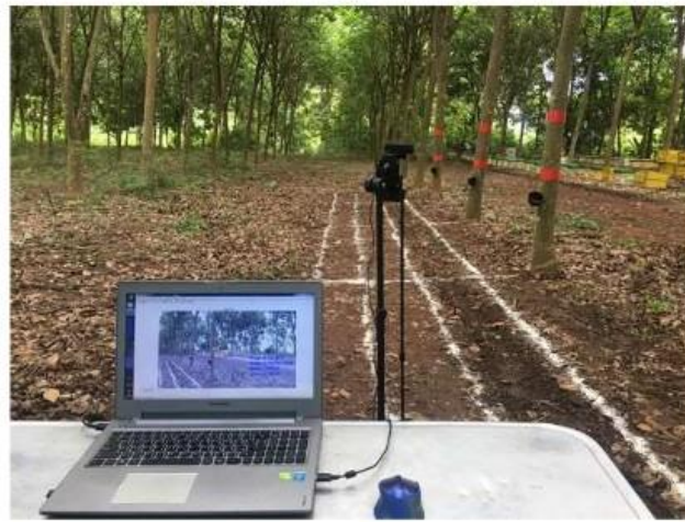
(a) Two separate targets on each rubber tree in an uncontrolled environment of an actual tree orchard
