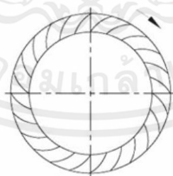
FORWARD CENTRIFUGAL BLADES FACING FORWARD TO DIRECTION OF ROTATION
