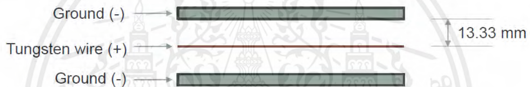
Figure 3.21 Configuration of Charging Electrode
