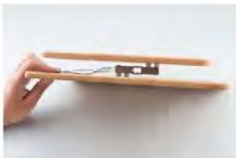
Bar load cell between a two plate configuration
