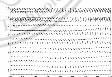
Fig. 15. vector field of velocities between groin when wavelength 0.5 \sin(t + 0.03x) .
