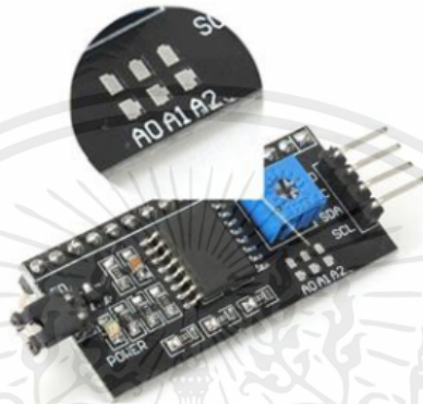
Address selection pads in the I2C-to-LCD piggy-back board.
