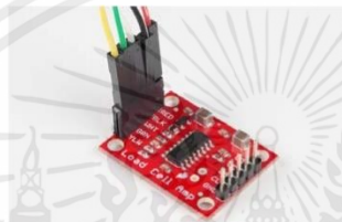
Load cell wires hooked up to the HX711 Amplifier board
