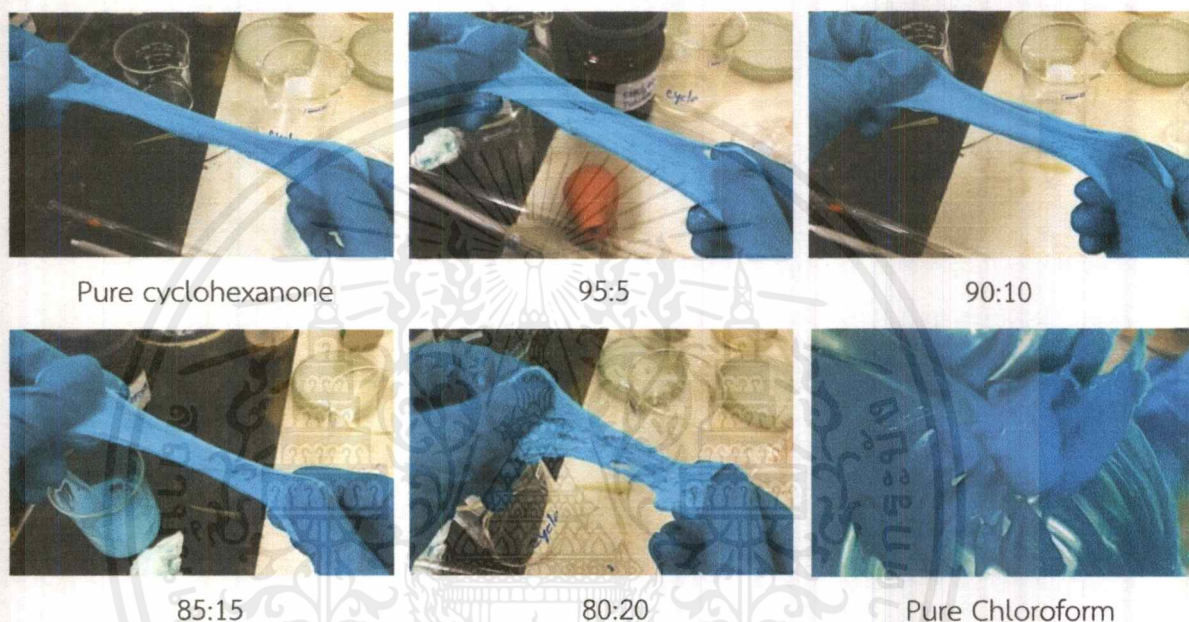
Figure 4.1 Coagulums of NBR latex compound by using different ratios of cyclohexanone and chloroform at 24 hr maturation time
