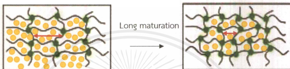
Figure 4.7 Increased crosslink density when maturation time was increased
