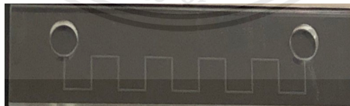
Figure 53 The device was bonded by magic tape.
