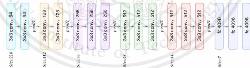
Figure 16. Structure of VGG-16
