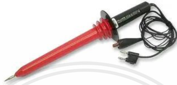
Figure 28. The high-voltage probe
