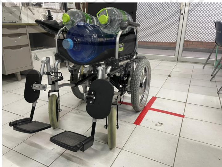
Figure 33. Notice angular calibration of wheelchair with loading weight.
