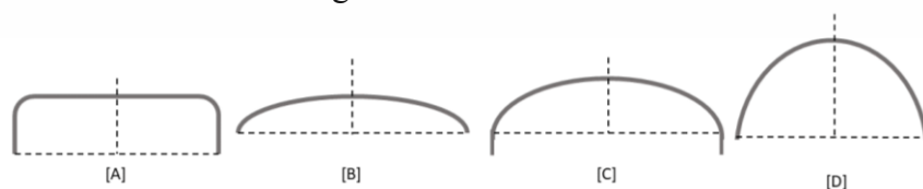
Figure 2.8: Types of cover and heads. Form head [A], torispherical head [B], ellipsoidal head [C] and hemispherical head [D] 20 .
