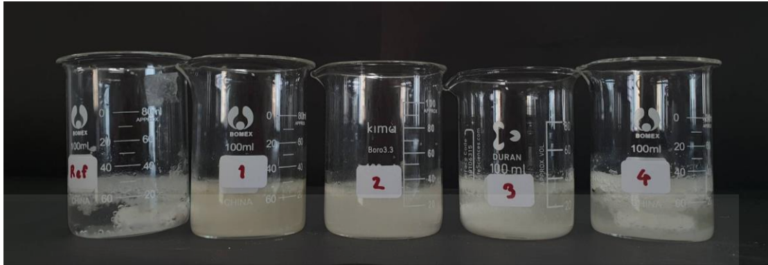
Figure38: The photo showing raft from each particle batches (from left to right: active ingredients, >1mm, 1mm-0.6mm, 0.6mm-0.45mm, <0.45mm)
