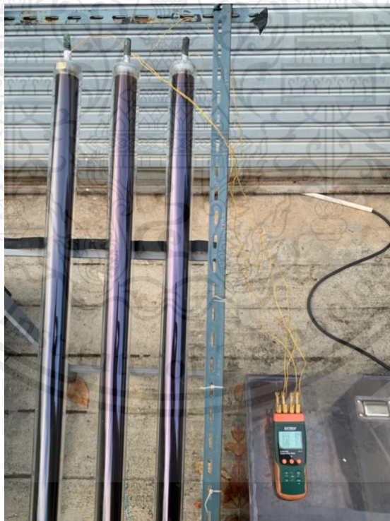
Figure 3.1: Evacuated tube solar collector with thermocouple and data logger
