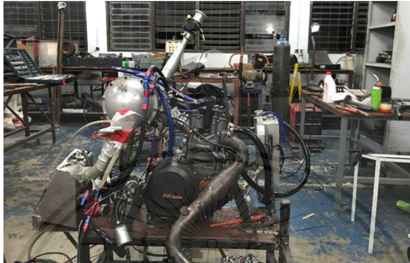
Figure 4.2 Assembly of the engine setup for intake system testing
