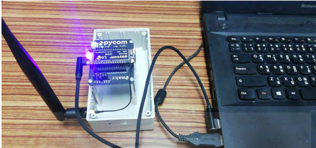
Figure 30: Testing of LoRa Gateway
