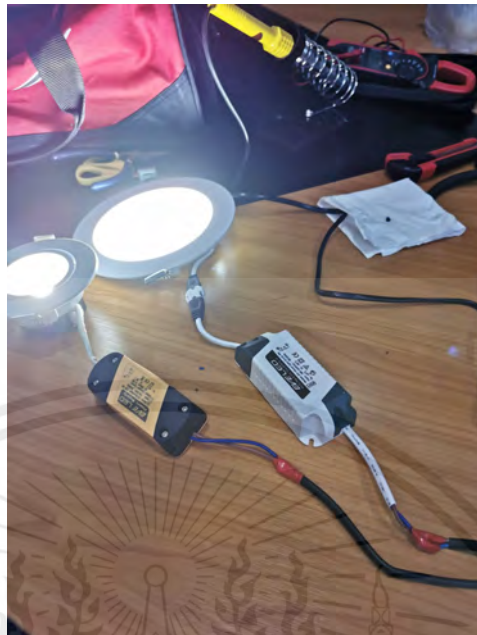
Figure 23: Modified LED panel and LED downlight
