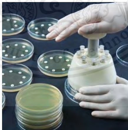
Figure 7: Automatic disc dispenser [14].
