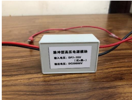
Figure 23. 20 kV high voltage generator used for generating the electrostatic field.
