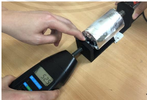
Figure 43. The average speed of the rotating collector is 52.5 rpm which is measured by the digital tachometer.
