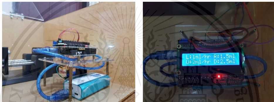
Figure 35. Controller of syringe pump
