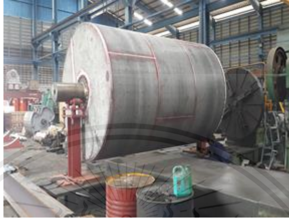
Figure 4.5: Mud Filter Drum
