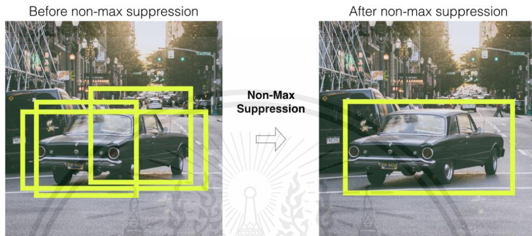
Figure 2.40 The non-max suppression process [36].
