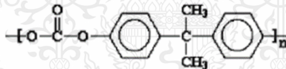
Figure 2.7 The repeating unit of polycarbonate [44].
