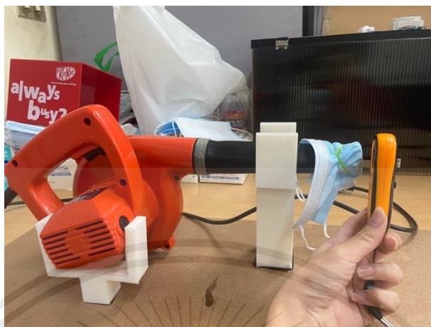
Figure 3.13 Experimental setup for air flow measurement
