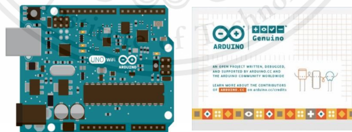
Fig.2.43 Arduino Board (left) and Arduino program (right) (Source: https://www.arduino-makerzone.com/article/1/arduino-basic-ep0-arduino-คืออะไรทำอะไรได้-มีกี่แบบ )
