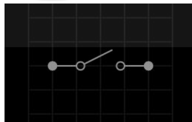
Fig.2.39 The SPST circuit symbol.
