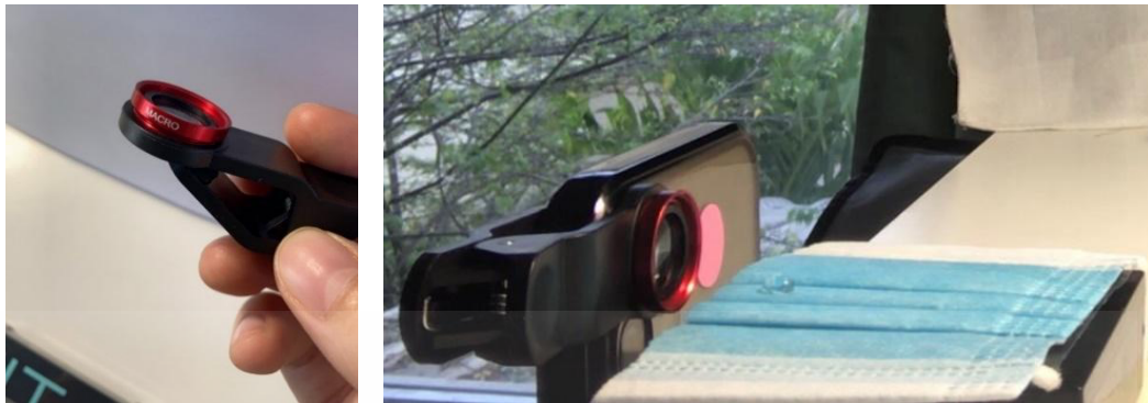
Figure 15. A macro lens clip (left) and the experimental setup with 2 cm distance between lens and the droplet (right)
