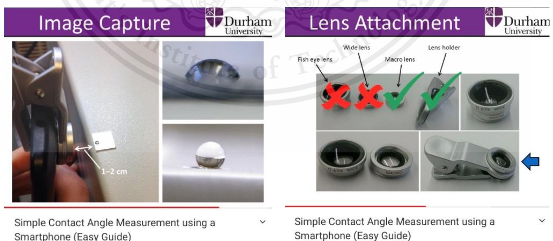
Figure 14. The reference methodology of a simple contact angle measurement using a smartphone [48].
