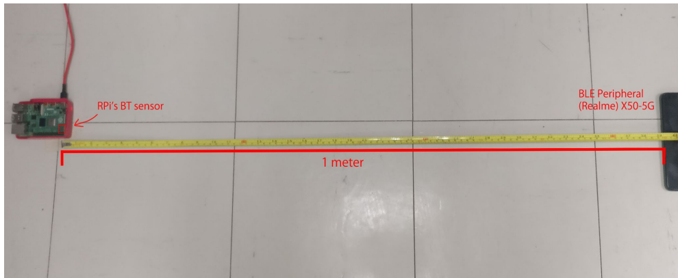
Figure 5.6: Peripheral Measured Power Calibration - (Realme) X50-5G
