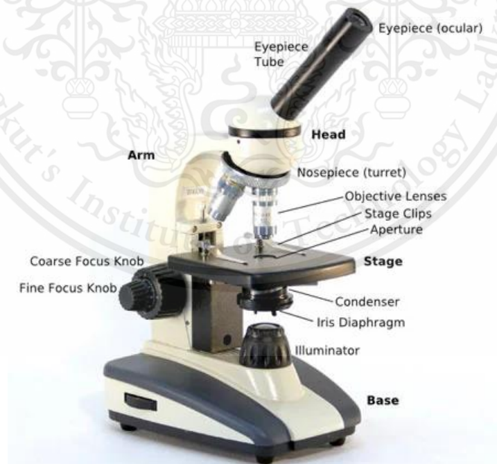
Figure 2.25: Optical component of optical microscope
