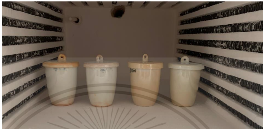
Figure 21: Convert powder of calcium by using High-Temperature Chamber Furnace
