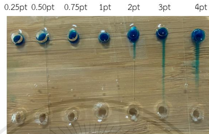
Figure 4.2 The liquid flowed through the 20 times printed layer channel of various width sizes of 0.25 pt to 4 pt
