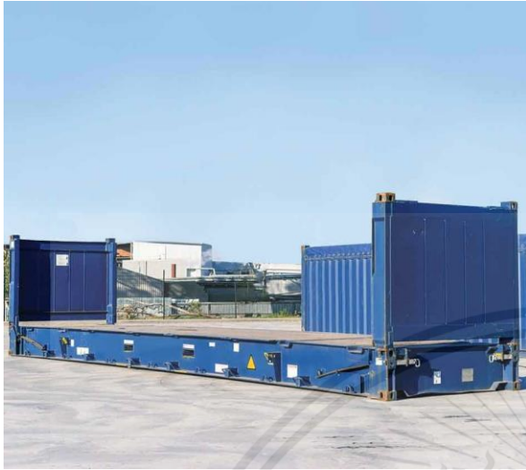
Figure 3: Flat Rack Containers
