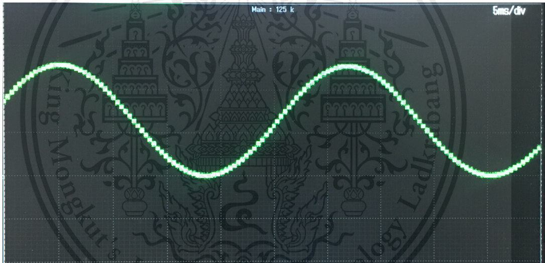
Figure 63 The results show the analog values convert from the MCP4725 board
