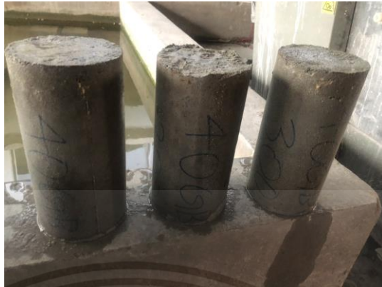
Figure 4.4 A cylinder concretes mixed fly ash.
