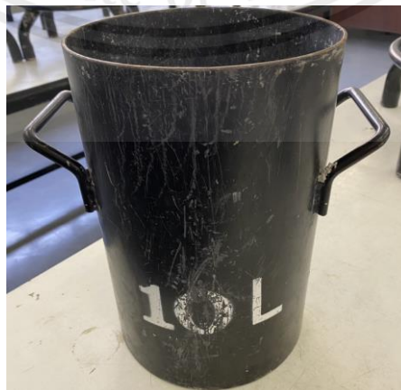
Figure 3.29 Smooth cylindrical container.
