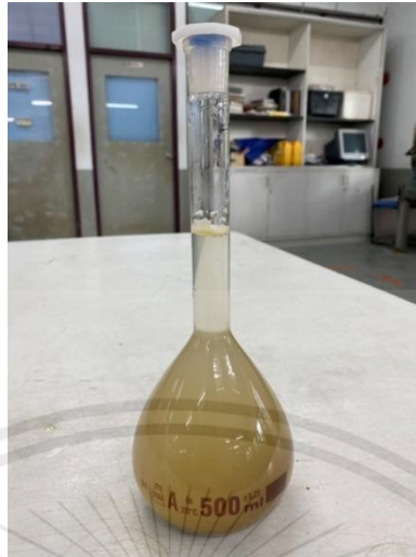
Figure 3.17 Fine aggregates in a volumetric flask.
