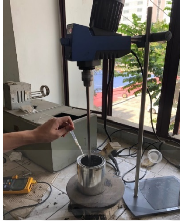
Figure 6. Mix asphalt binder with plastic.
