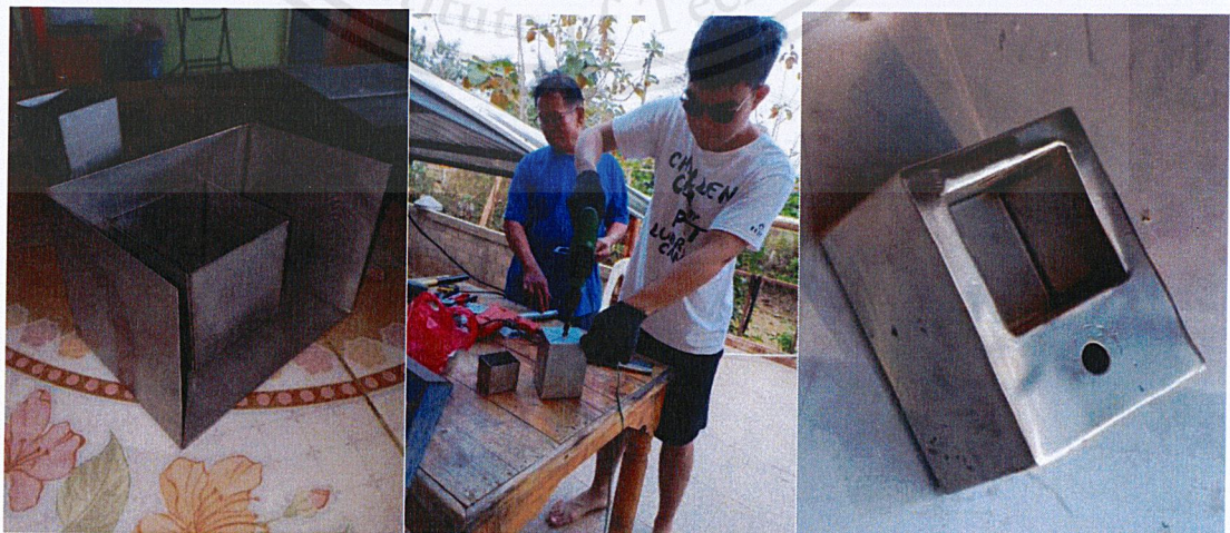
Figure B3: The Assembly of Evaporator part
