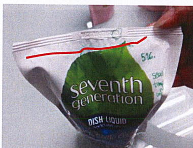
Figure 4.2: Sealing defect at Front
