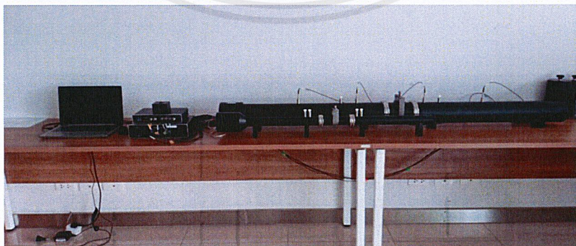
Figure 3-4: Impedance tube system in testing room.
