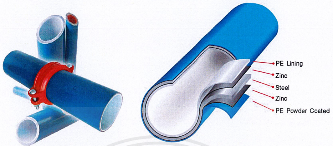
Figure 4.6 Polyethylene-lined steel pipe (sylene pipe)
