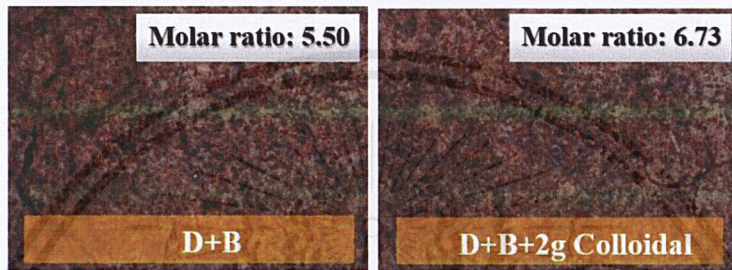
Figure B.5 Optical microscope of the film-forming of the samples (filler D+B).
