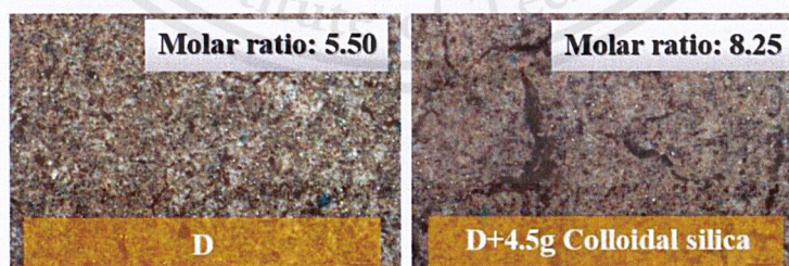
Figure B.3 Optical microscope of the film-forming of the samples (filler D).
