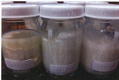
Figure A3 2 M. NaOH gives the best results to preventing the coagulation in the natural rubber.
