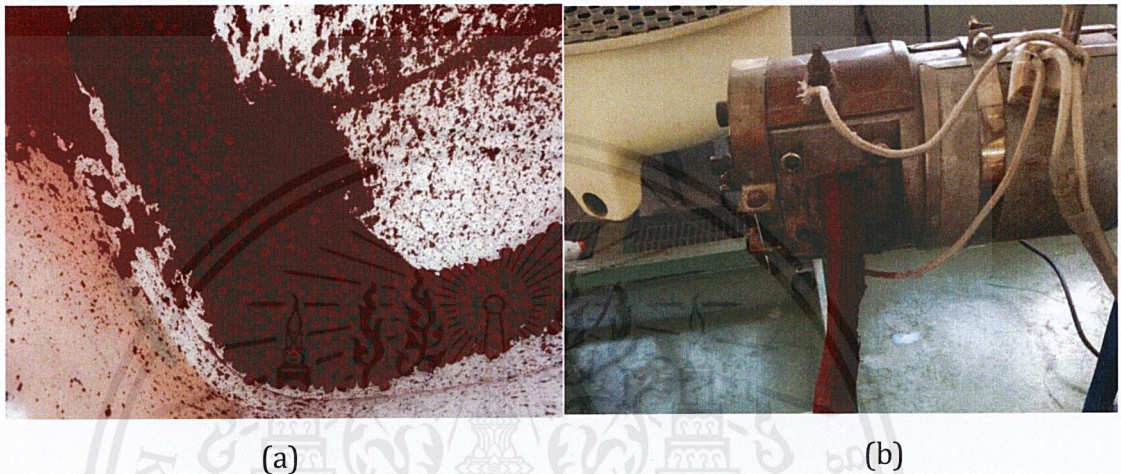
Figure 3.6 (a) LDPE beads and \text{Fe}_2\text{O}_3 powder compounding in a bucket and (b) twin screw extruder
