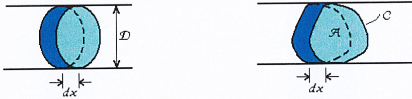
Figure 2.5 Control volumes for the analysis of fully developed flow in circular pipes and non-circular ducts
