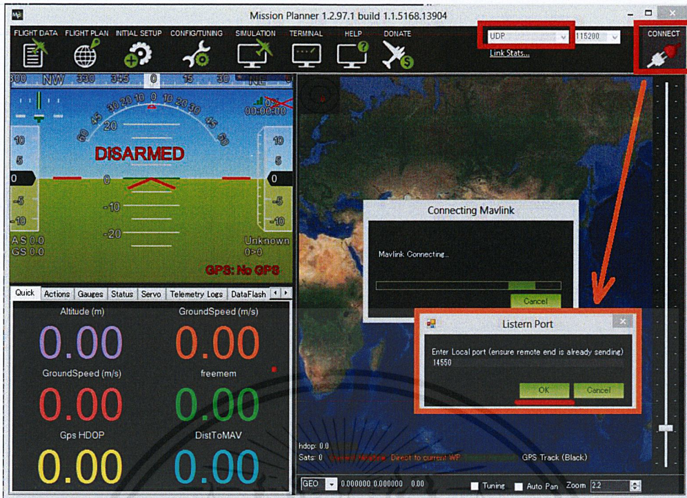
Figure 3-13. Mission Planner software for Pixhawk and drone setup, control, monitor, calibration.
