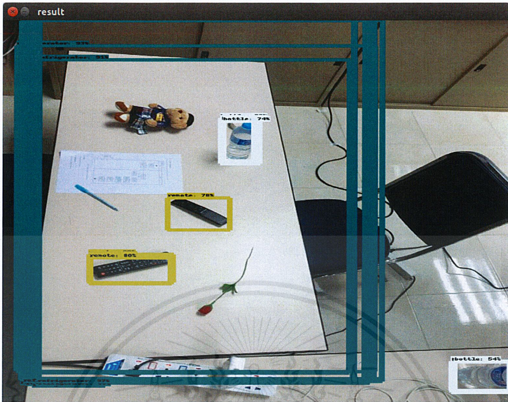
Figure B-27. Classification result using Faster R-CNN ResNet-101 model.
