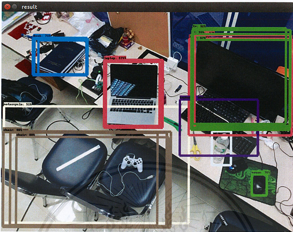
Figure B-35. Classification result using Faster R-CNN ResNet-101 model.
