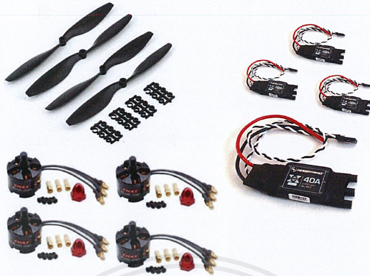
Figure 3-6. This figure includes the propellers, four EMAX MT2213-920KV brushless motors, and four 40A ESCs without BECs.
