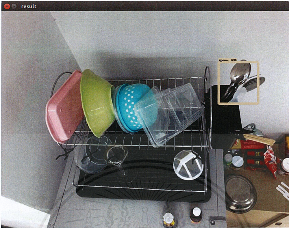
Figure B-4. Classification result using Faster R-CNN Inception v2 model.
