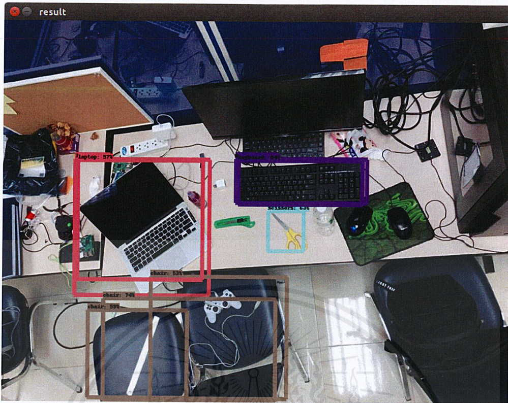
Figure 5-4. Classification result using Faster R-CNN Inception v2 model.
