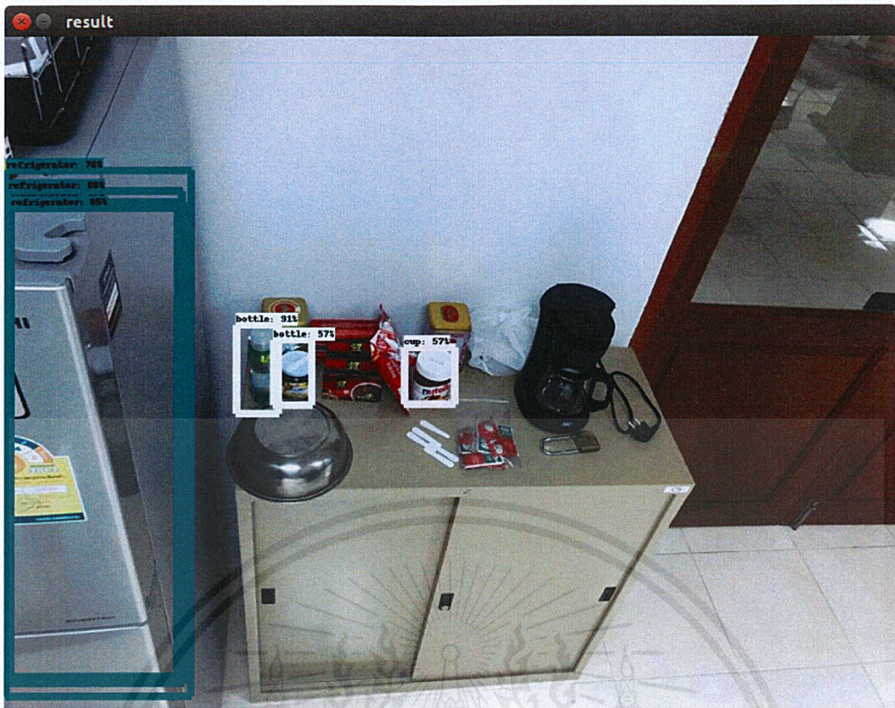
Figure B-20. Classification result using Faster R-CNN Inception v2 model.
