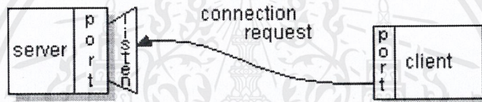
Figure 2-33. Client request for connection.
