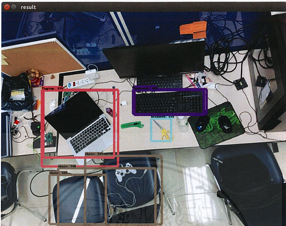
Figure B-40. Classification result using Faster R-CNN Inception v2 model.
