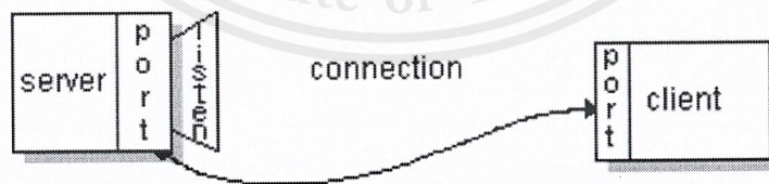
Figure 2-34. Connection being made.
